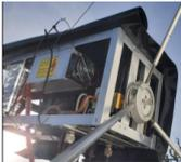
DL7YC's resized 47 GHz TWT (42 W) Hughes 8901MA at feed of his 2.4 m dish - note the size of the actual feed.
