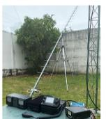
TICSDA operated 432 in EME Contest with 22 of HB LFA yag and 180 W
