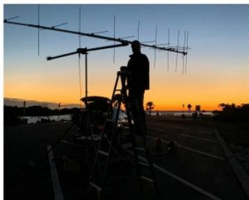
K6GU in EL89, setting up the antennas on a parking lot at the ocean with the sun setting behind him. Later Peter had to move the fully assembled array (~70 kg weight) closer to the water, right next to the palm tree in the background. In a second run he then had to carry the 200 kg of cement blocks that support the antennas down there.
