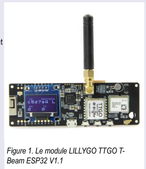
Figure 1. Le module LILLYGO TTGO T-Beam ESP32 V1.1
