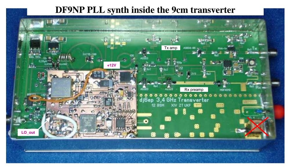
The DF9NP LO output is soldered after the strap desoldering (page 27)
