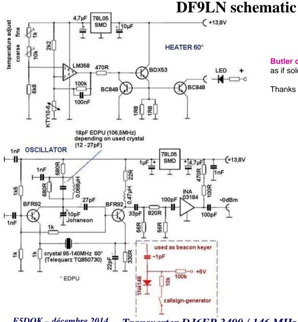
Butler oscillator with far better phase/noise behaviour as if soldered inside the transverter
