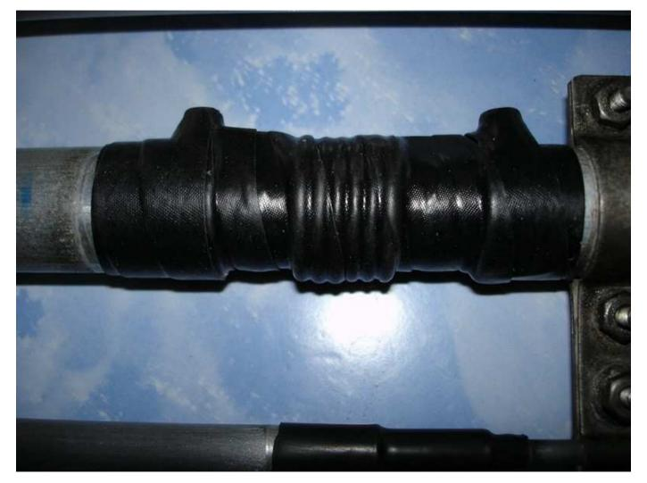
Application on 15 meter coil. Ensure that Alu tube must be sealed to the epoxy one
