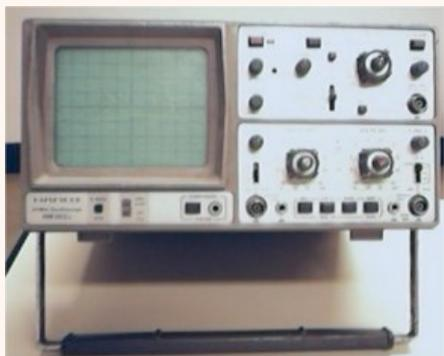
Oscilloscope 2 x 20 MHz
