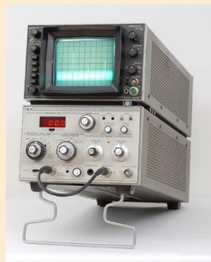
**Analyseur de spectre Hewlett Packard, HP 8558B HP181T (1973-1975) (Source Internet HP memory Project).**
